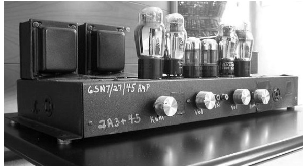
Figure 5: 1 Watt Single Ended Triode Amplifier
