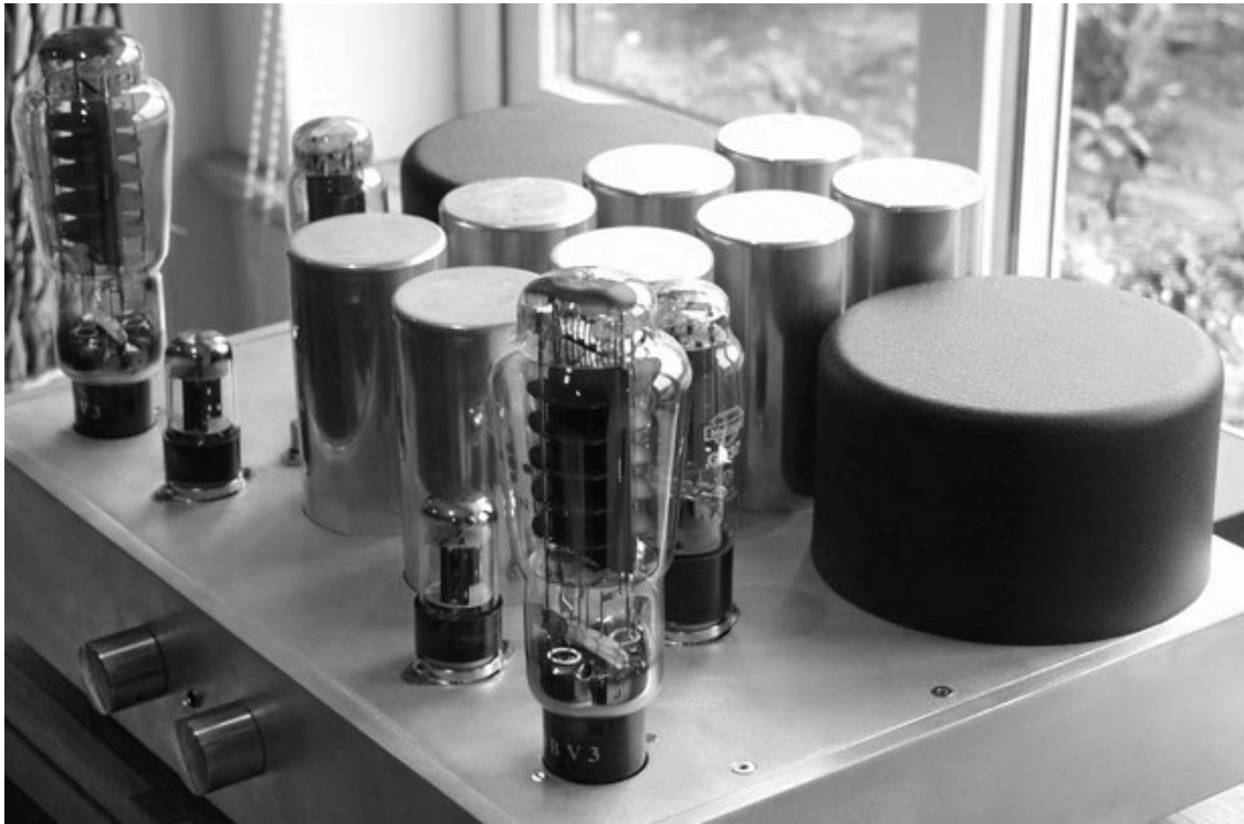
Figure 3: 20 Watt Single Ended Triode Amplifier
