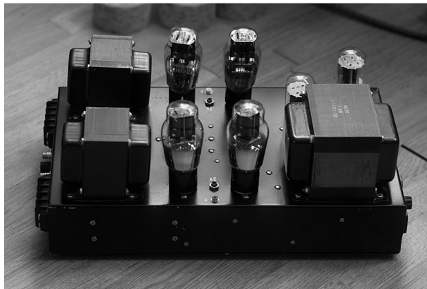
Figure 1: 8 Watt Push Pull Amplifier
